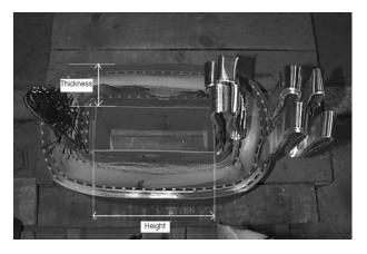
**Figure 1** Hybrid coil manufactured with circular copper conductor in the high-voltage winding and aluminium foil in the low-voltage winding This winding is called low-high-low (LHL)
