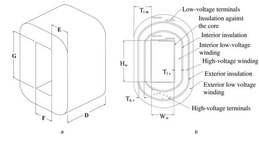
**Figure 8** Active part of single-phase shell-type transformer *a* Core dimensions
