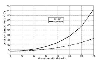
**Figure 4** Average temperature against current density for copper and aluminium under a short-circuit condition with duration of 4 s
