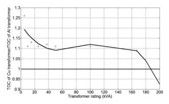
**Figure 5** Ratio of TOC (\$) of copper transformers over TOC (\$) of aluminium transformers as a function of transformer rating (kVA)
