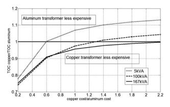
**Figure 6** Ratio of TOC (\$) of copper transformers over TOC (\$) of aluminium transformers as a function of the ratio of copper unit cost (\$/kg) over aluminium cost (\$/kg) for 5, 100 and 167 kVA single-phase transformers
