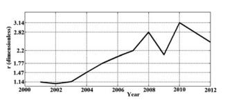
**Figure 2** Ratio of copper unit cost over aluminium unit cost, *r*, from 2001 to 2012
